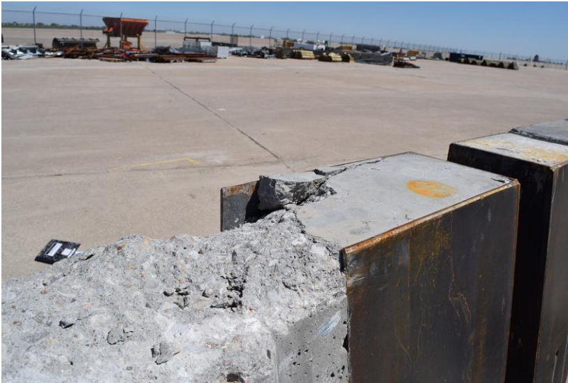
Figure 42. System Damage, Cover Plate Removed, Test No. MAN-1
