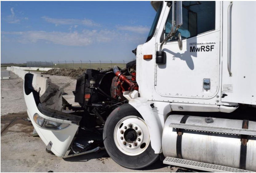
Figure 44. Vehicle Damage, Test No. MAN-1
