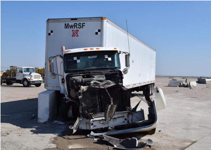
Figure 45. Vehicle Damage, Test No. MAN-1
