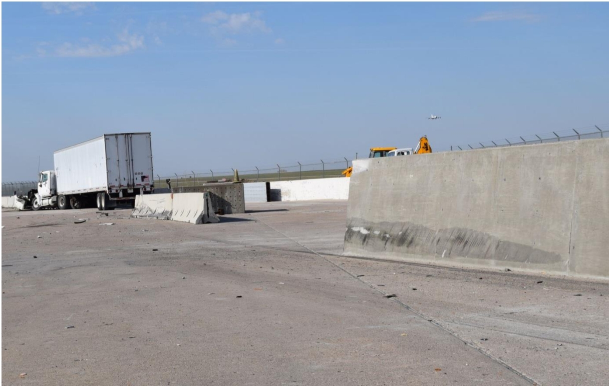
Figure 39. Vehicle Final Position and Trajectory Marks, Test No. MAN-1
