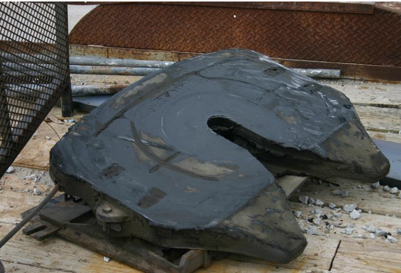
Figure 46. Fifth Wheel Plate Damage, Test No. MAN-1
